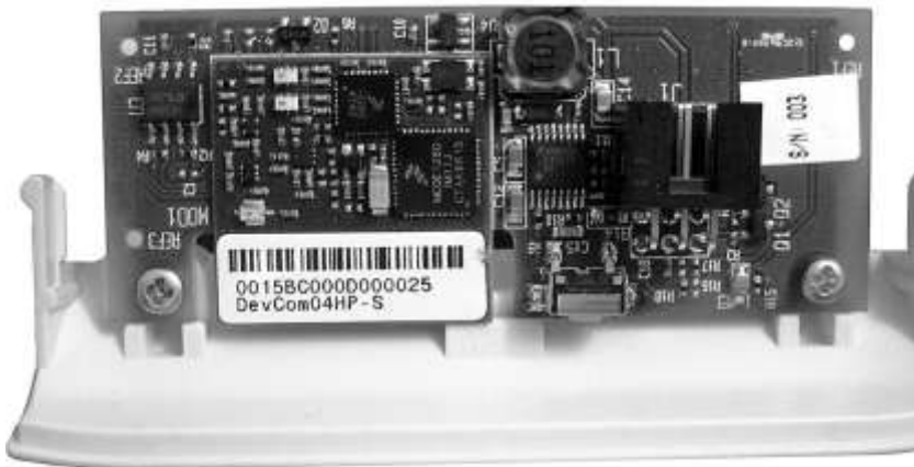
Fig. 3–8. A PLC-RF bridge device deployed in Europe. (Photo by Dorthe Gaardbo-Pedersen; courtesy of Develco.)
