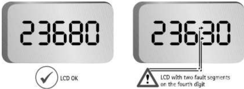
Fig. 4–10. An example of display failure
