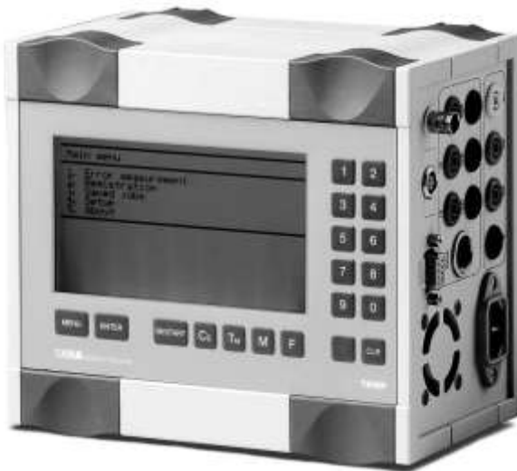
Fig. 1–32. Example of a metering test device. (Photo courtesy of Iskraemeco.)
