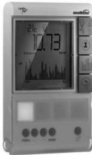
Fig. 3–9. A smart customer display unit deployed in Oceania. (Photo courtesy of Landis+Gyr.)
