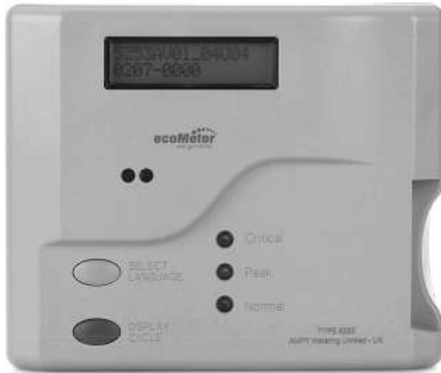
Fig. 1–23. A customer display unit. (Photo by Landis+Gyr.)
