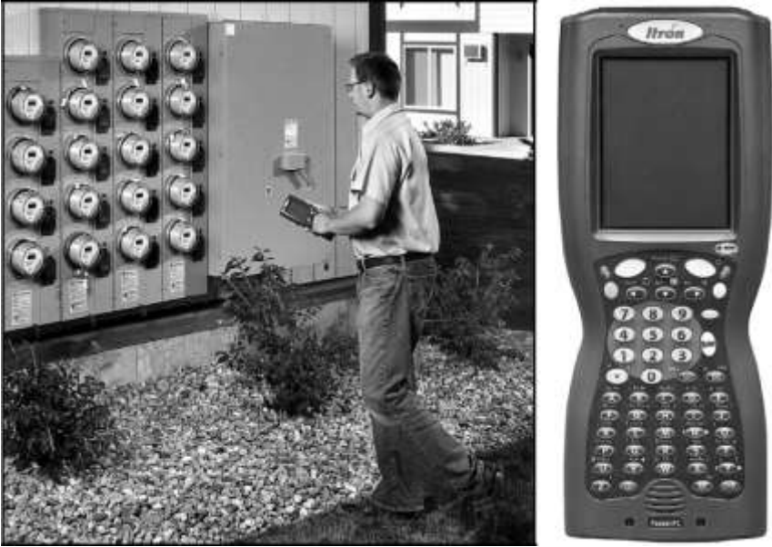
Fig. 1–30. A special handheld unit used for walk-by services. (Photo Courtesy of Actaris.)
