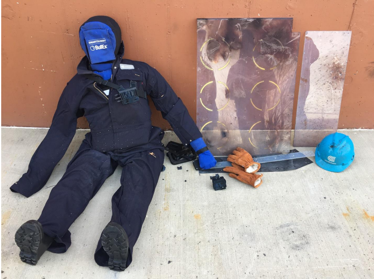
Aftermath of Arc Flash DNV-GL Test of the Cubicle Inspection & Repair Safety Device Figure 7
