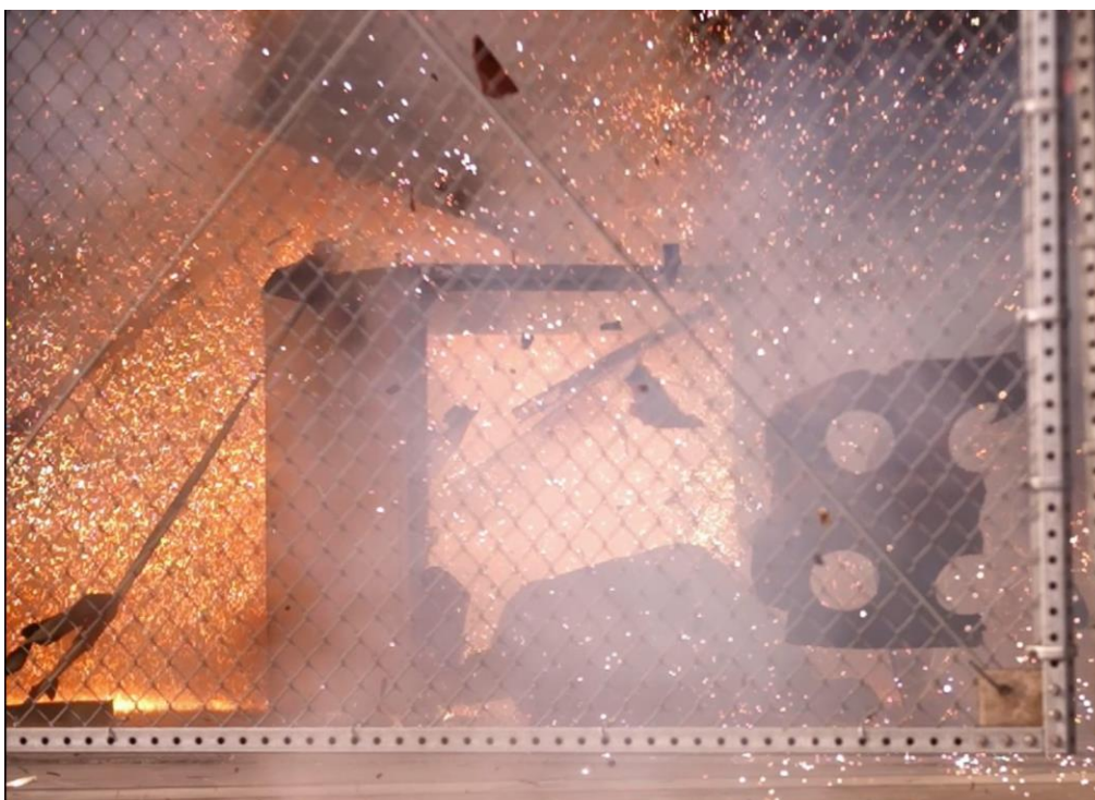
Photo during Arc Flash DNV-GL Test of the Cubicle Inspection & Repair Safety Device Figure 6
