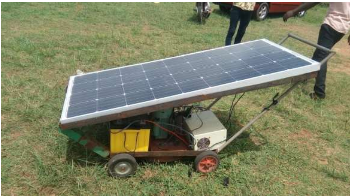
Figure 1: The fabricated solar powered lawn mower
