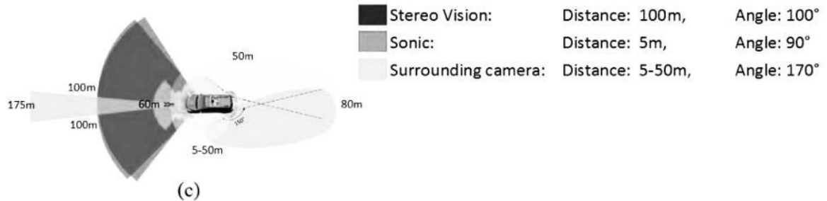
Fig. 7: Sensor ranges and distances. Different shades stand for different sensors. Source: [15].
